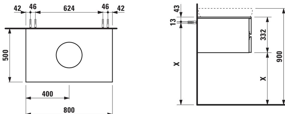
X = The exact height must be set during installation.
