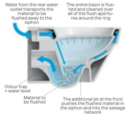
A new type of WC having highest-performance flushes with volumes of 4.5 and 6 litres. This unique model unites all worldwide standards. Maximum performance tests have shown that this powerful WC is prepared to meet future standards. It does already achieve outstanding flushing results with 2-3 litres, if the downstream drainage systems are designed for this purpose.
